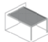
Pared Portería lama paralela a pared On facade Louvers parallel to the wall
